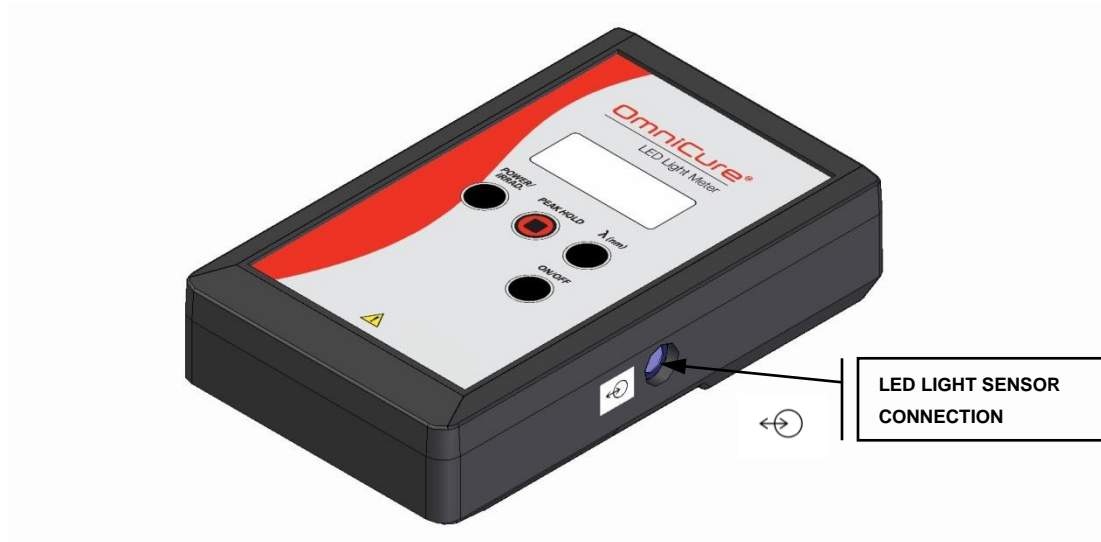
Figure 2 LED Light Sensor Connection
