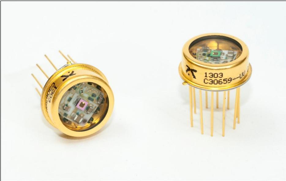
*Excelitas' C30659-UV-1 APD Preamplifier Module enables high responsivity at 500 nm and offers a very low noise floor.*
