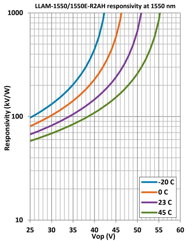
Si and InGaAs Low-Light Analog APD Receiver Modules (LLAM)
