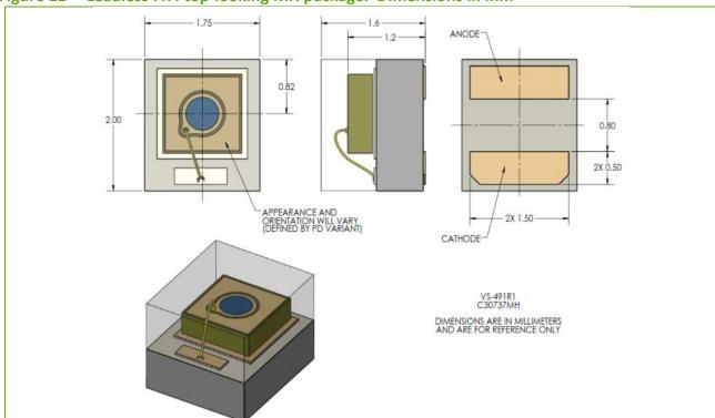
Figure 11 – Leadless FR4 top-looking MH package. Dimensions in mm
