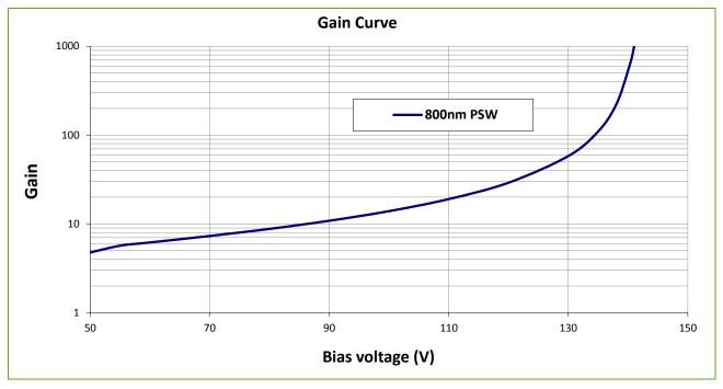
Figure 6 – Typical gain vs. bias voltage for 900nm peak sensitivity wavelength types
