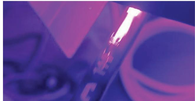
Many UV-curing systems have used high-intensity lamps as a UV source. But lamp-based systems have a number of disadvantages including high power consumption, high cost of operation and maintenance and the need for ventilation to remove ozone from the work area. These lamps also generate and deliver heat to the curing site, which can cause product shrinkage and deformation.
