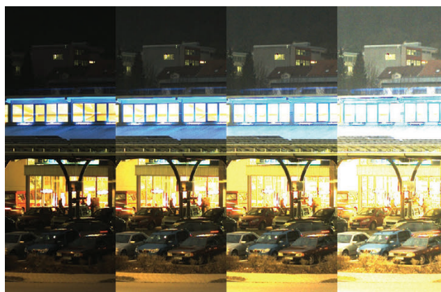
Figure 1: Four extracts of the same night image, which was taken one evening outside the lab of a supermarket in Kelheim using a pco.edge 5.5 color sCMOS camera system. Each image demonstrates how the 16 bit image was scaled to the 8 bit world of the print or the screen, but all versions have been created from the same raw data file. The image on the left side shows a full scale conversion (value 65536 (16 bit max) -> value 256 (8 bit max) and value 0 (16 bit) -> value 0 (8 bit)), while image on the right shows a low scale conversion (value 1024 (16 bit low) -> value 256 (8 bit max) and value 0 (16 bit) -> value 0 (8 bit)). The other images show different conversions in between.
