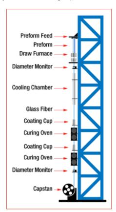
FIGURE 1: Schematic of a fiber optic drawing tower.
