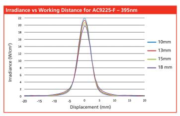
Typically, an LED curing system is very sensitive to the working distance, where the irradiance level will change significantly with small changes to the working distance. The custom optics of the OmniCure AC9225-F system maintain the irradiance almost unchanged from 10 to 18 mm, the typical working distances for the fiber coating application.
