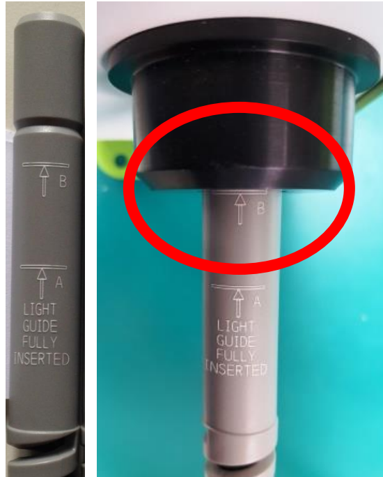
Figure 4 Correct position for fully inserted X-Cite LLG and LLG with A and B insertion lines
